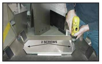
**Figure 7.1** For top vent, remove the two screws holding the top heat shield in place. For rear vent, see Section 7B.
